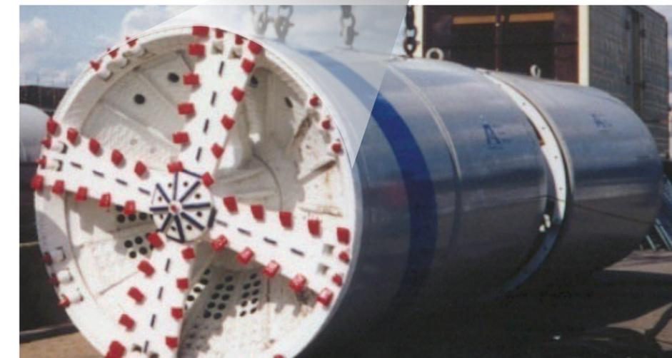
A cutterwheel excavates material at the face of the machine, as shown in Figure 2. A sophisticated laser system ensures that the tunneling operation continues at the correct angle.
