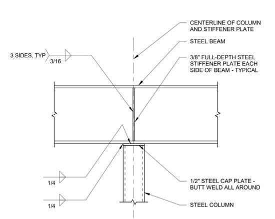
**206 STEEL BEAM TO STEEL COLUMN CONNECTION**
