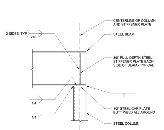
**204 STEEL BEAM TO STEEL COLUMN CONNECTION**
